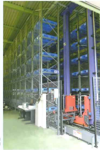
金型・材料自動収納庫 The storage warehouse for die mold in which die mold pattern is placed automatically and neatly
